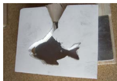
Fig. 2 Styrene board mold
