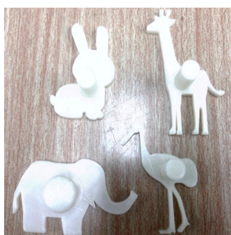
Fig. 4 Stamp produced by 3D printer
