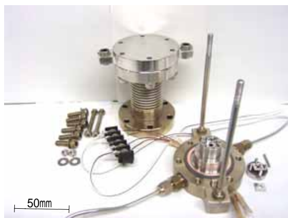
Fig. 2 SP test jig equipped with formed bellows.
