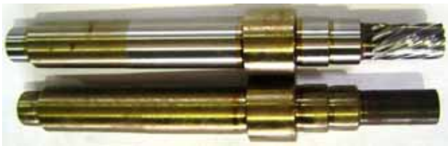
Fig. 8 Before and after RGC method of motor shaft for gear motor
